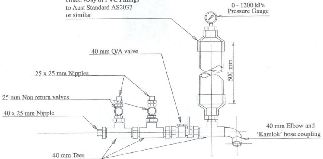
Hint: Use rigid PVC/Polythene/Brass fittings where possible to avoid corrosion problems.
